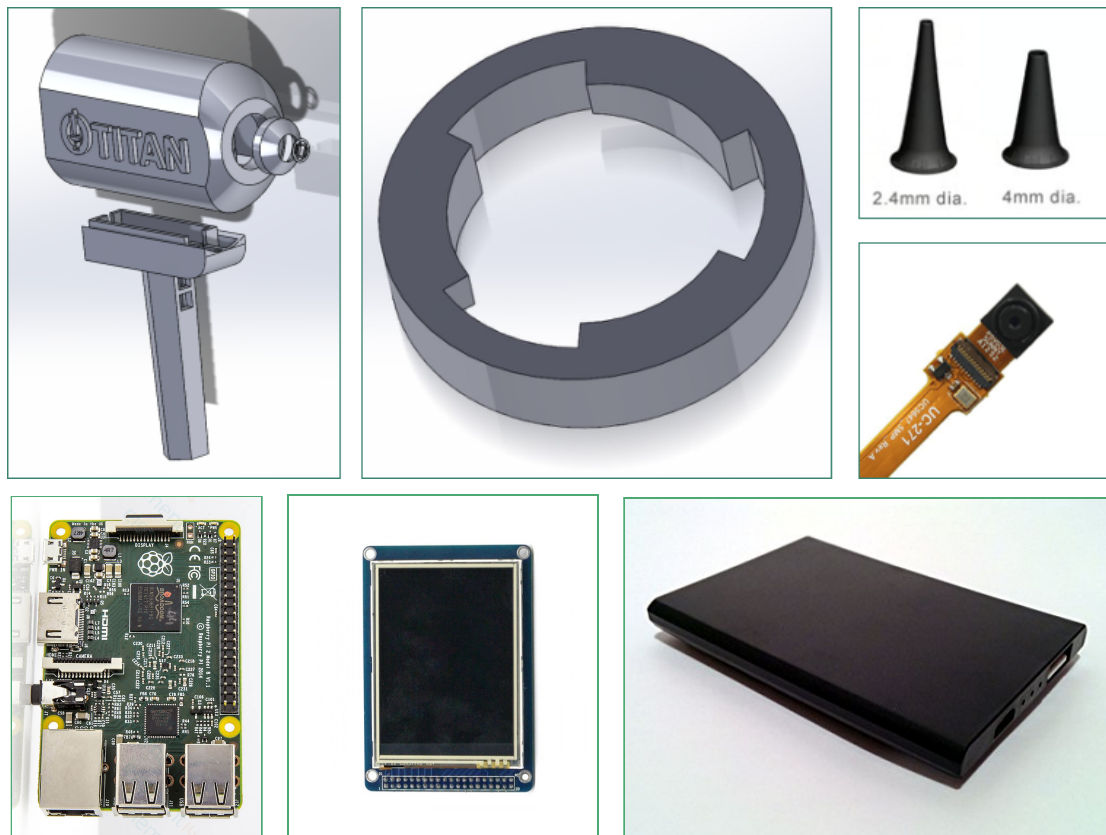
Figure 32. The components in the final AURI prototype. From left to right is the final prototype, the ear specula securing ring, disposable ear specula of different sizes, the Raspberry Pi Spy Camera, the Raspberry Pi processor, the display monitor, and the rechargeable battery.
