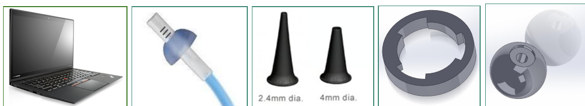
Figure 27. The components in AURI. From left to right are the controller/processor, the camera, different sizes of speculum, the ring for securing the speculum onto the handle, and the handle.
