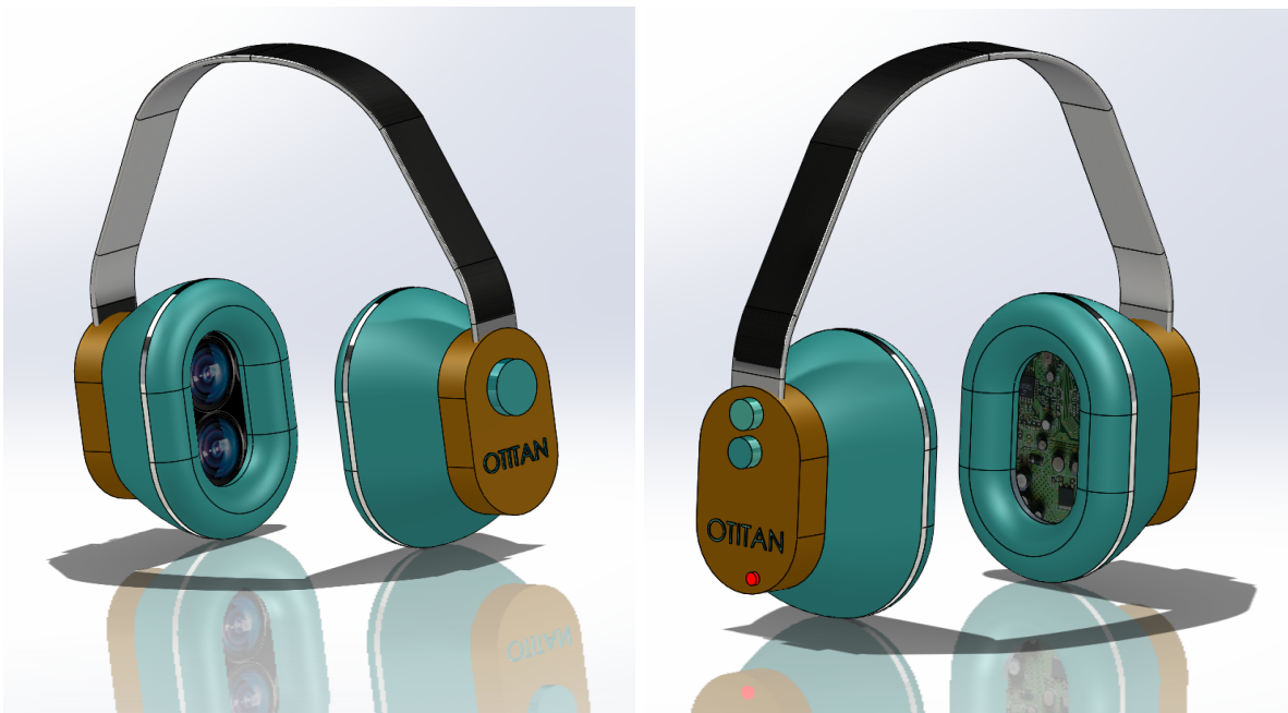
Figure 12. Over-the-ear prototype of prospective solution with an integrated camera for image acquisition (left) and a circuit system to test for fluid viscosity (right). Although shown separately, both components will be included together on both sides of the device.
