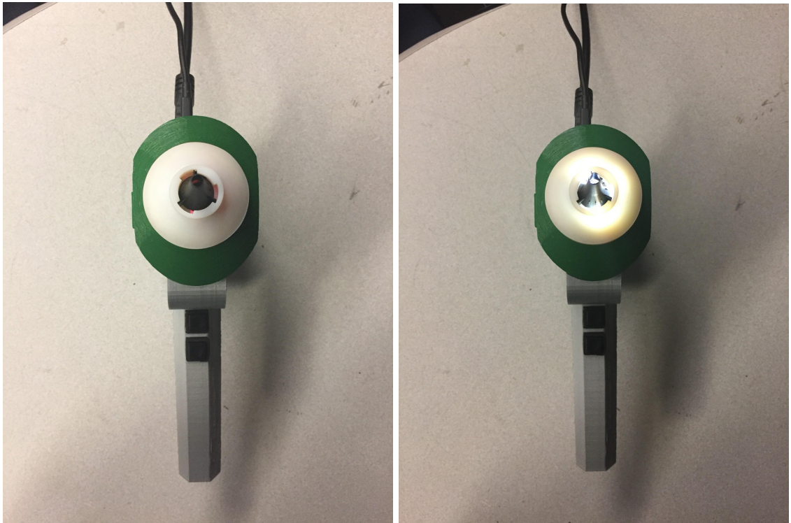
Figure 36. Images showing the lighting system for the spy camera. The left shows when the lighting system is off, while the right shows when the lighting system is on.
